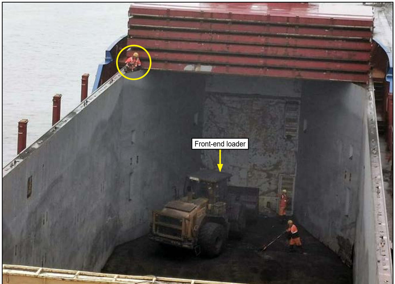
Figure 8: Photograph taken by ship's crew after the cargo operations resumed, showing stevedores working in the forward end of the cargo hold with a stevedore coordinator sat on top of the cargo hatch coaming
