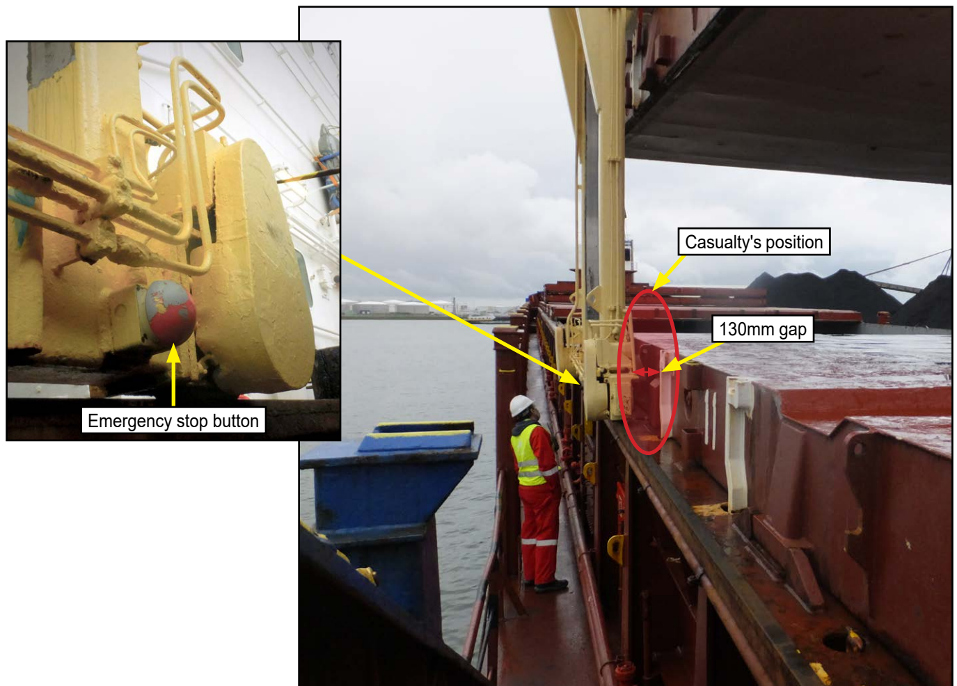
Figure 6: View of location where stevedore coordinator was discovered with inset showing position of emergency stop button
