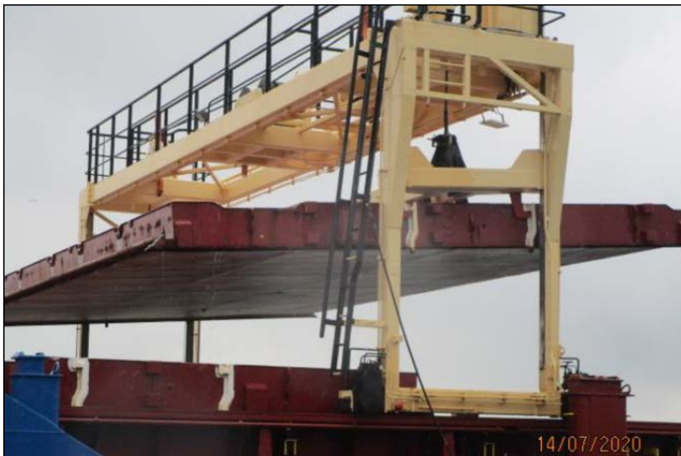
Figure 5: Gantry crane (in accident position) with hatch cover 9 suspended
