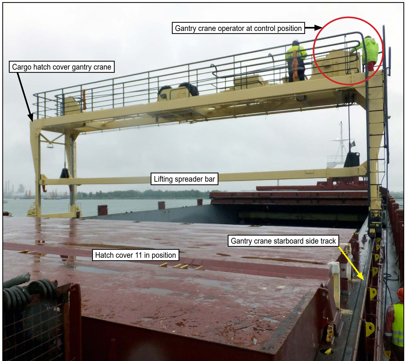
Figure 1: Cimbris ' hatch cover gantry crane (photograph taken from the vessel's starboard side, looking forward)
